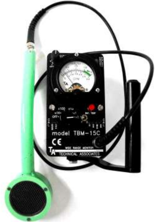
TBM-15 WITH GM PROBE
