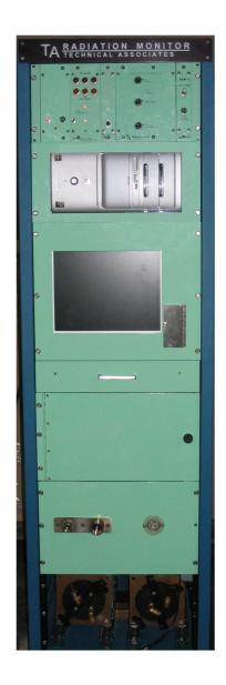
The entire system is mounted in a self-contained rugged cabinet and comes complete with all cabling, connectors, and software in place, setup, and ready to operate. The standard unit is operated from 115 V single phase, 60 Hz; 220V optional, 50 or 60 Hz.
