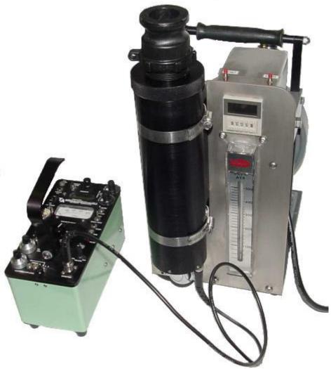
**APPLICATION:** The FR Series Air Monitor assures Safety against airborne Radon or other radioactivity contamination by means of constant check with alarm and optional record capability. It provides integrated exposure information. The FR Series is sensitive and versatile. Although designed as an industrial workplace and hospital breathing air measurement system, it may be used to monitor Radon in any medical, industrial or residential setting down to EPA levels.
