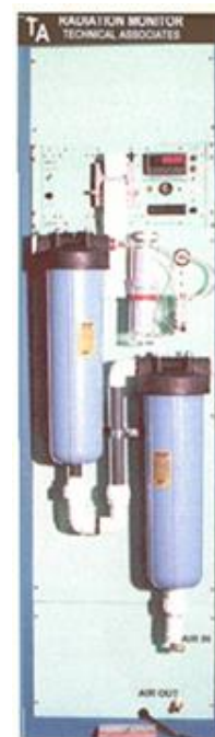
EXTERNAL CABINET VIEW FILTERS ON OUTSIDE
